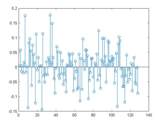
Filter the transmission data through an AWGN channel with minimal noise. OFDM reception reverses the transmission processing. Apply an FFT and QAM demodulation, and then confirm that the received symbols match the transmitted symbols.
