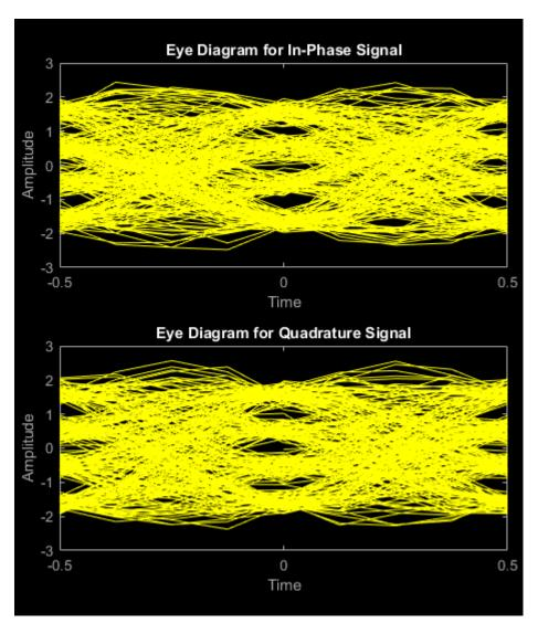
Displaying the eye diagram of the signal after the receive filtering is applied shows the signal with raised cosine filtering. The wider eye diagram eye-openings, the signal has less ISI with raised cosine filtering as compared to the signal with RRC filtering.
