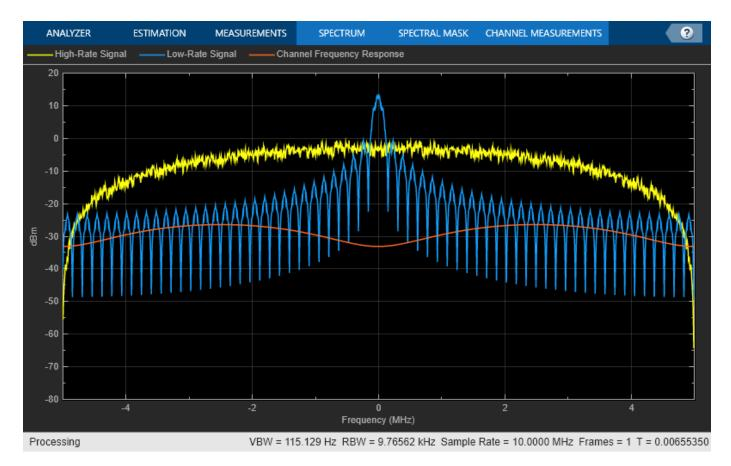
To avoid ISI while transmitting many parallel low bandwidth signals, the individual subcarriers must be orthogonal to each other. Avoiding ISI by transmitting many orthogonal low bandwidth subcarriers motivates OFDM. An OFDM modulator converts a high-rate serial stream of symbols into many parallel low-rate streams. Each orthogonal low-rate stream encounters a relatively flat channel with minimal ISI, and can be easily equalized.
