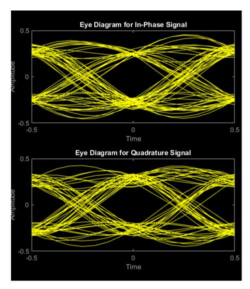
Display 1000 points of the received signal eye diagram.
