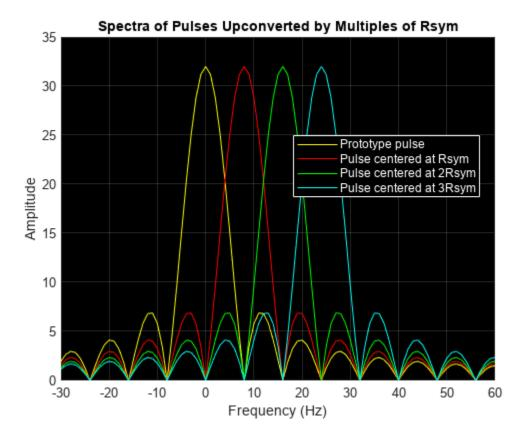
The frequency domain plot shows the orthogonal frequency translated pulses with spectral peaks of each subcarrier occurring at the zero crossings of all the other pulses.
